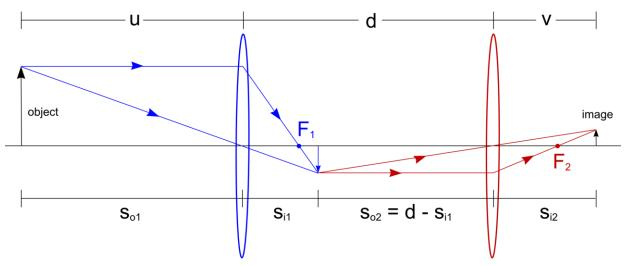
Design Specs: You are to find the focal lengths  $f_1$  and  $f_2$  of the two 2 thin lenses shown above, where u = 6 ft, d = 10 ft, v = 4 ft, and the magnification is + 1 /36. In this way, a child 36 inches tall (object) will have a corresponding image size of 1 inch projected on the glass viewing screen!
