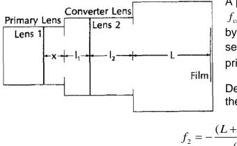
A primary camera lens with focal length  $f_{\text{camera}} = f_1$  can be converted into a telephoto lens by inserting a diverging lens, the converter secondary lens with focal length  $f_2$ , between the primary lens and camera body.
