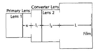
A primary camera lens with focal length  $f_{\text{camera}} = f_1$  can be converted into a telephoto lens by inserting a diverging lens, the converter secondary lens with focal length  $f_2$ , between the primary lens and camera body.
