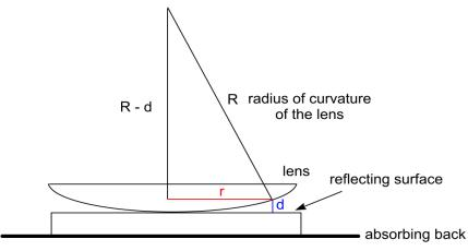
A lens sits on a flat reflecting surface. Take R to be very far away. Then, light traveling downward reflects partially at the back curved surface of the lens while the some light passes on and reflects off the optical flat. We will consider these two as the main beams.
