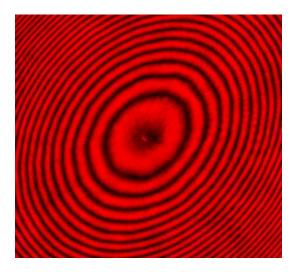
"Newton's rings interference pattern created by a plano-convex lens illuminated by 650 nm red laser light, photographed using a low-light microscope. The illumination is from above, leading to a dark central region." Wikipedia: Robert D. Anderson. Creative Commons
