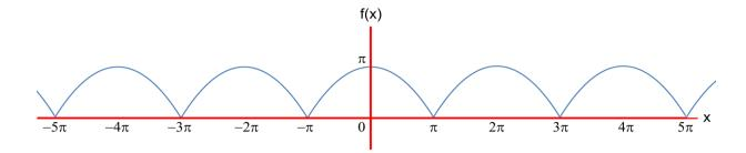
The periodic wave shown above is a repeating section of an inverted parabola.
