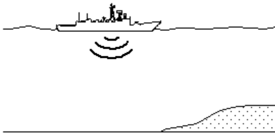
Fig. D-1. SONAR: Sound Waves Used to Measure the Depth of Water.
