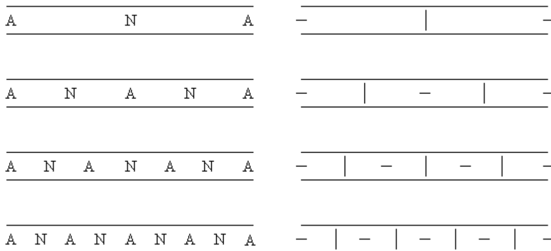
Fig. H-7. The First Four Standing Waves in an Open Pipe Defined by Displacement.
