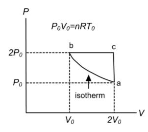
**HW-G3.** Simple Engine With Isotherm. An engine with an ideal a-b-c cycle.
