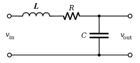
Your impedances are  $Z_L = j\omega L$ ,  $Z_R = R$ , and  $Z_C = \frac{1}{j\omega C}$ , where  $j = \sqrt{-1}$ . From your transfer function  $H(\omega)$  find the relative transmission  $|H(\omega)|$ . Show that the charge q(t) on the capacitor for an input voltage  $V_{in}(t) = V_0 \sin \omega t$  is given by
